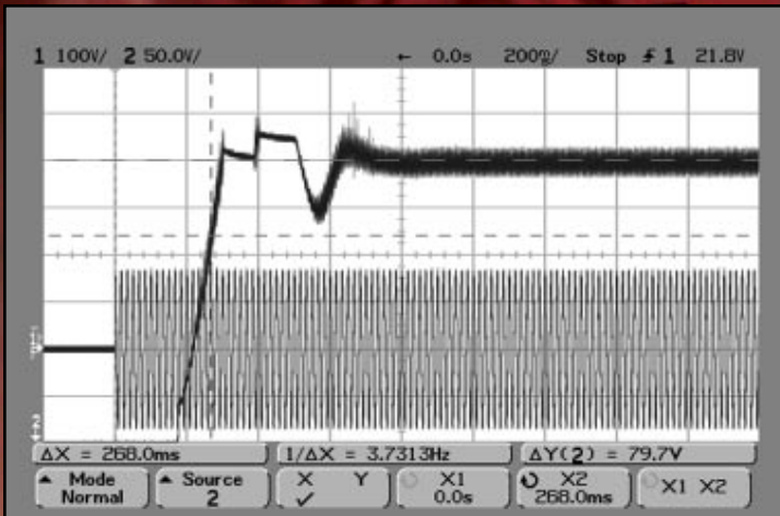
TURN ON TIME 940 \mu\text{F} , 25°C, 500W
